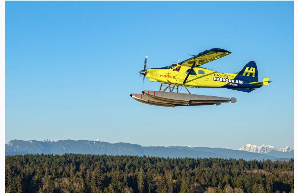
Harbour Air's electric DHC-2 proof-of-concept prototype, dubbed the eBeaver. Harbour Air Photo
